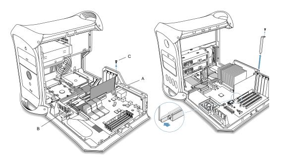
2. If you are removing a PCI video card, gently pull up the card and remove it from its PCI expansion slot.
